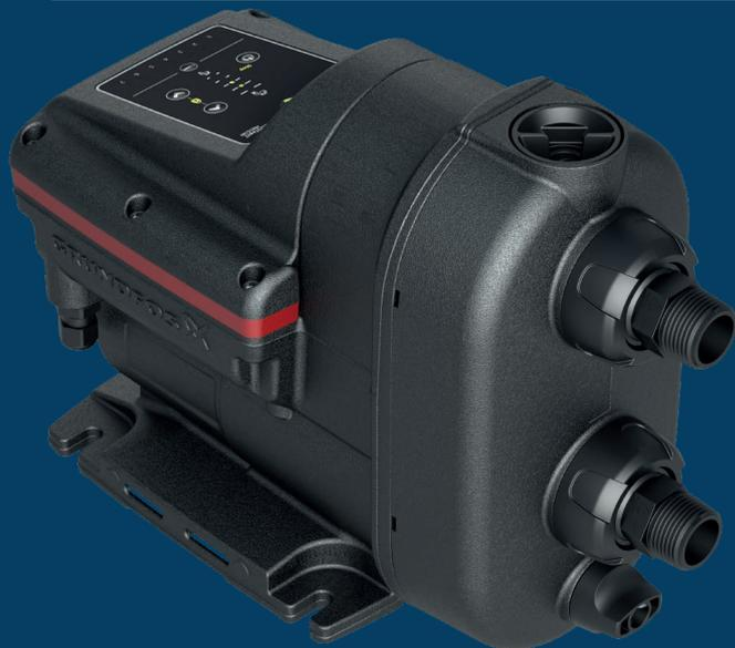
GRUNDFOS SCALA2 is a robust, composite, variable speed pump that adjusts performance according to water demand, providing constant pressure to all taps. The fully integrated pump includes a motor, tank, sensor, drive and non-return valve in one compact unit that is quick and easy to install. The SCALA2 is self-priming, allowing for use from both above and below ground water sources and the water-cooled motor ensures quiet operation.
